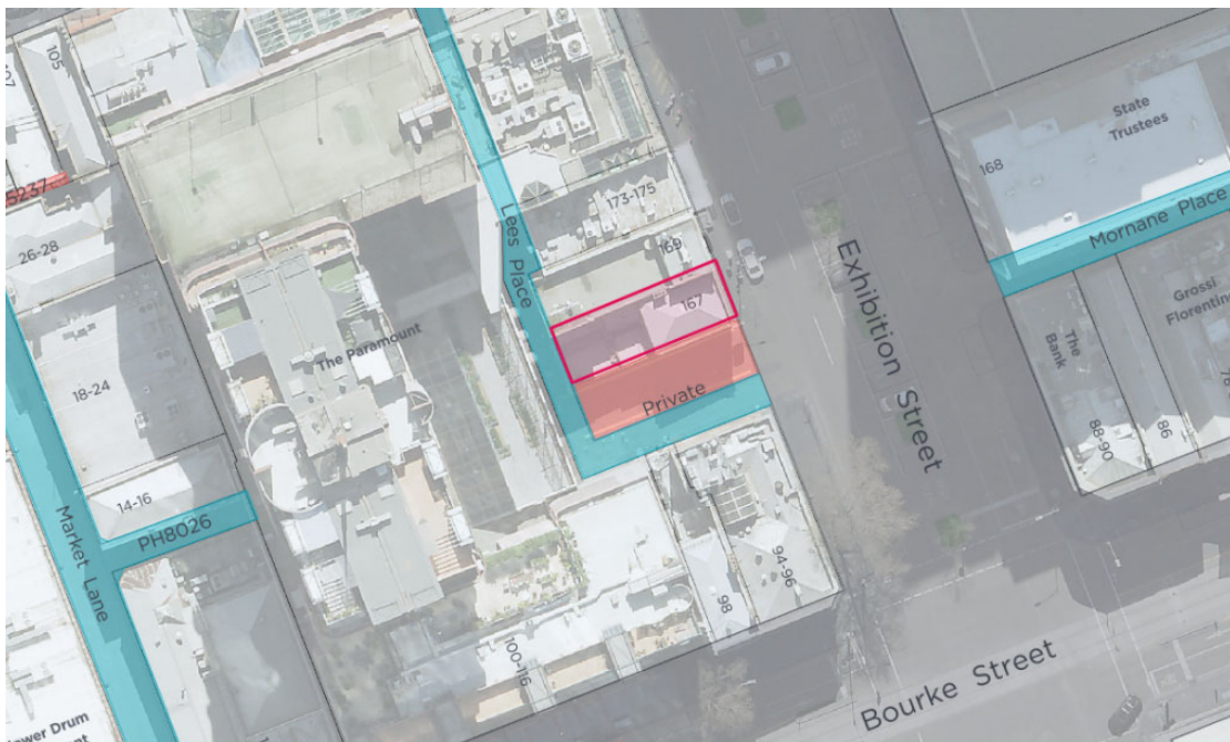
Figure 2 – Aerial image of subject site and status of abutting laneways (private laneways shown in red and public laneways shown in blue)
