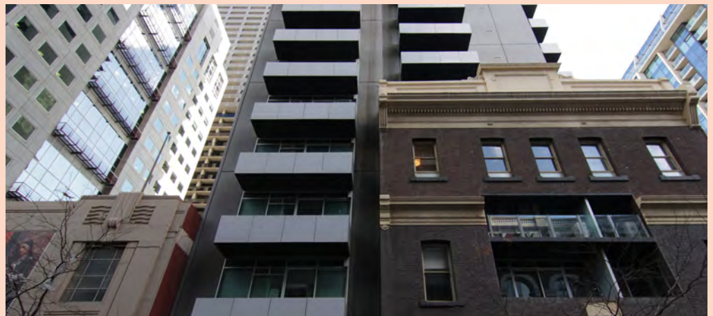
Figure 28 The alignment of balustrade banding is insufficient to create a successful massing relationship to the retained heritage form.
