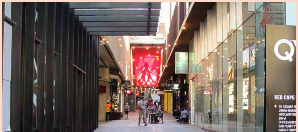
Figure 78 Canopies that cover the majority of a laneway reduce the sense of openness and publicness, while obscuring any visual connection to upper levels.
