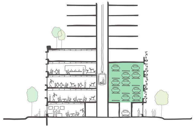
Figure 40 The structure of the building, including the design of the floorplate and positioning of openings is designed to accommodate habitable spaces in the future.
