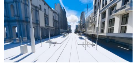
Bourke Street Mall Stage 2 – extract from survey accuracy electronic model being for the Vehicle Barrier Design
