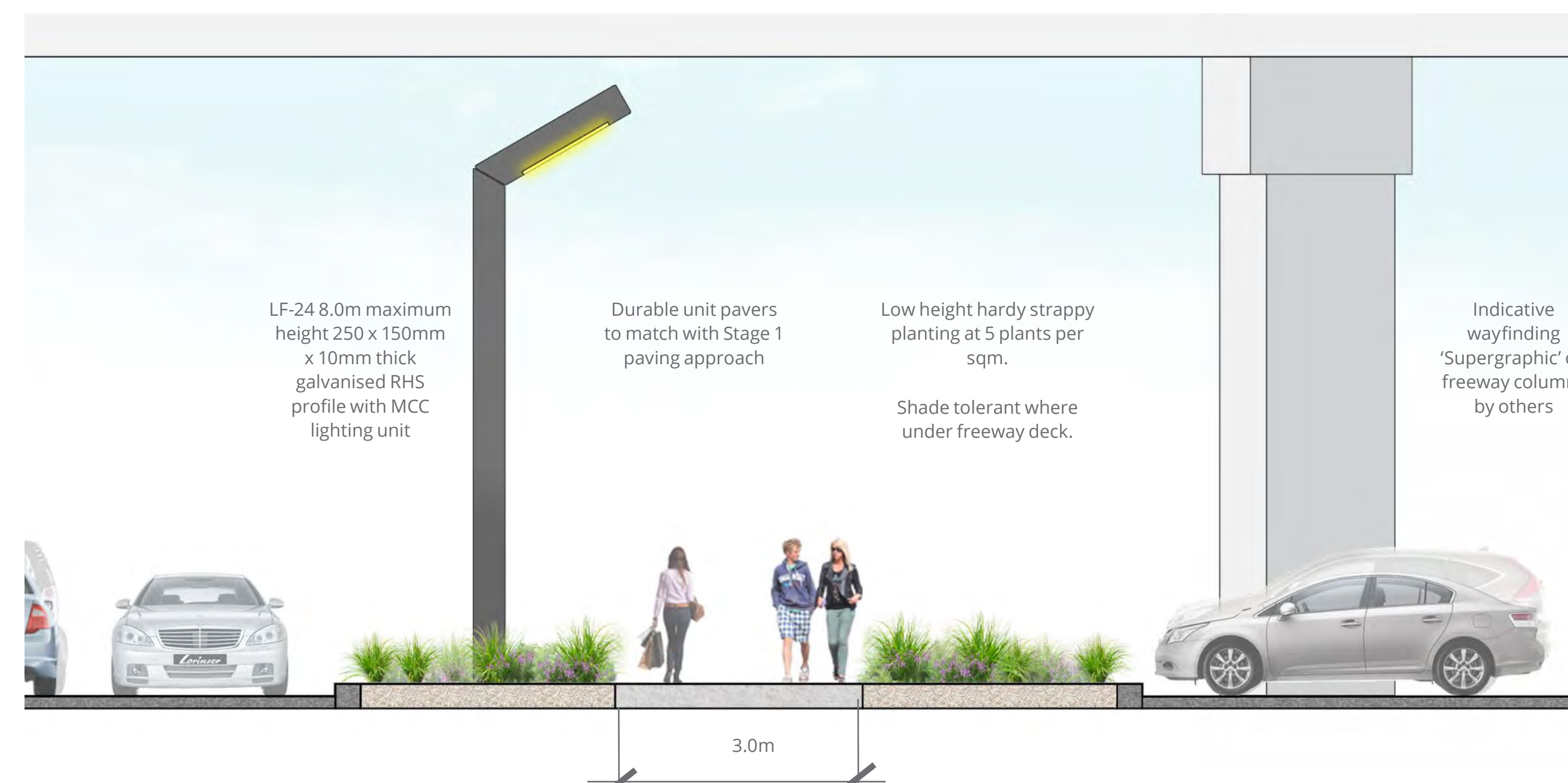
INDICATIVE SECTION THROUGH PEDESTRIAN PATH
