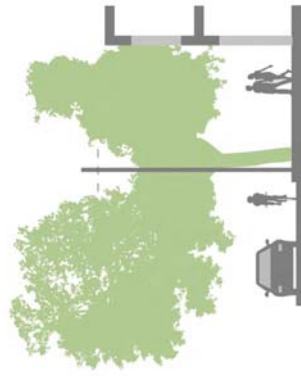
Tree trimmed under powerlines
