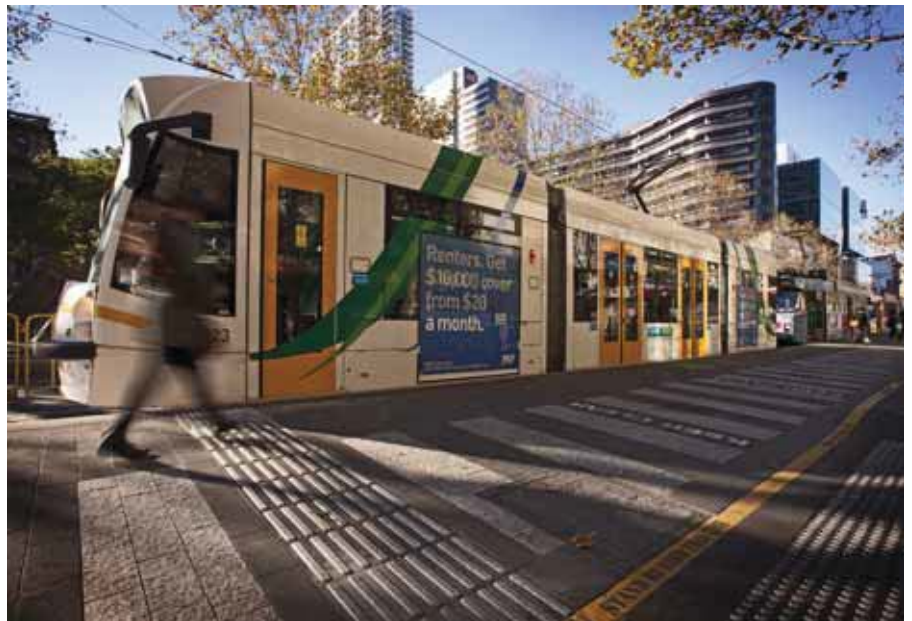
Fig 7.1 Level access tram stop in Swanston Street, Melbourne
