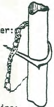
Round Downpipe: Spike Fixing
