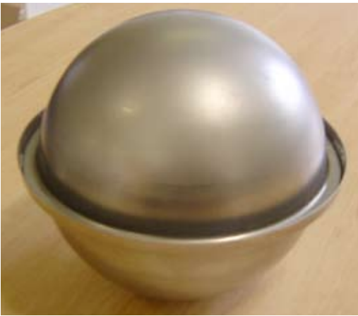
Figure 5. Final option for housing the phase change material
