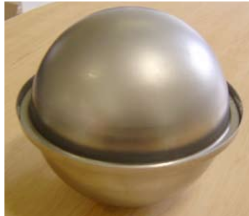
Figure 1. Final PCM storage vessel
