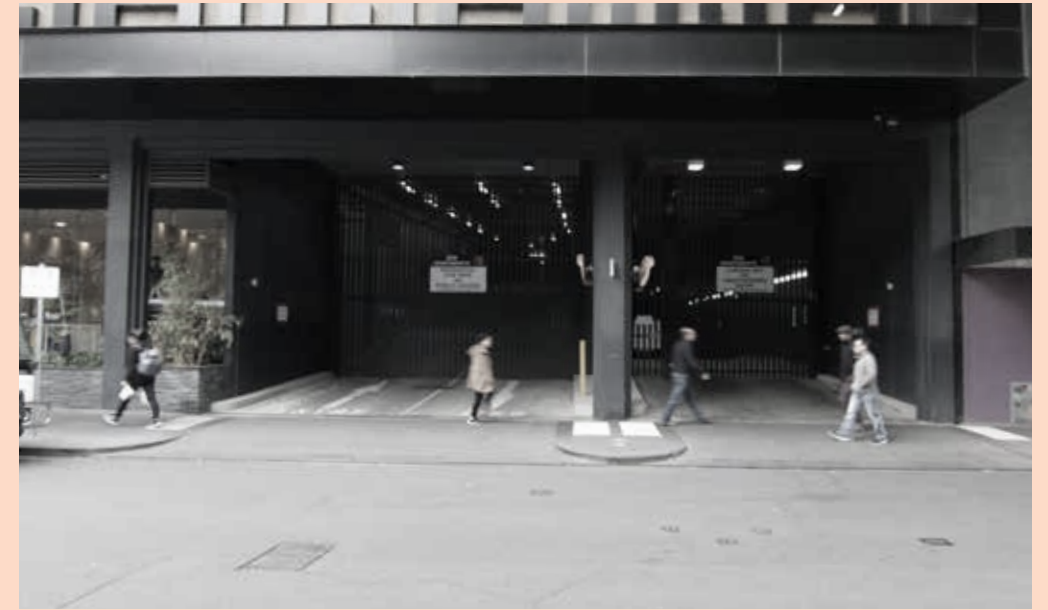
Figure 38 A deep setback to the carpark access door results in an undesirable space which feels unsafe at night and impacts the continuity of the pedestrian realm.
