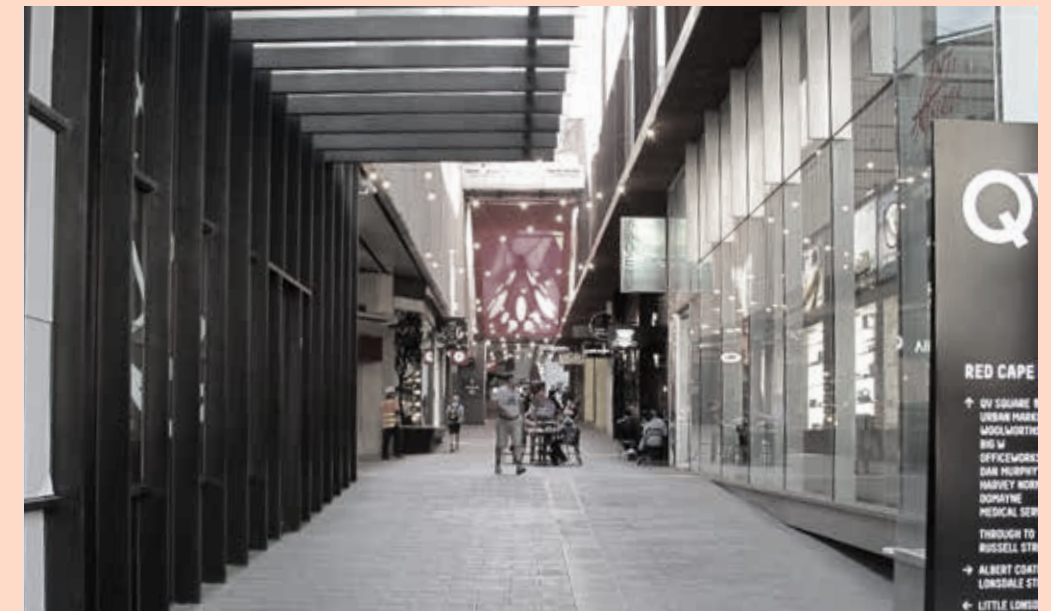
Figure 49 Canopies that cover the majority of a laneway reduce the sense of openness and publicness, while obscuring any visual connection to upper levels.
