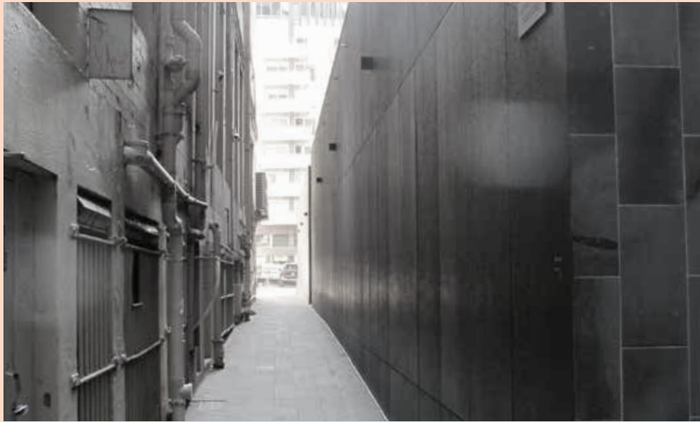
Figure 7 Blank walls along a public connection reduce the safety and usability of the space
