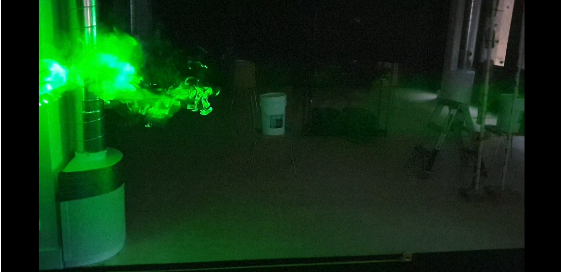
FIG. 24. Simulated cough in Displacement Ventilation. Note that the smoke here extended approximately 2 metres from the source location.
