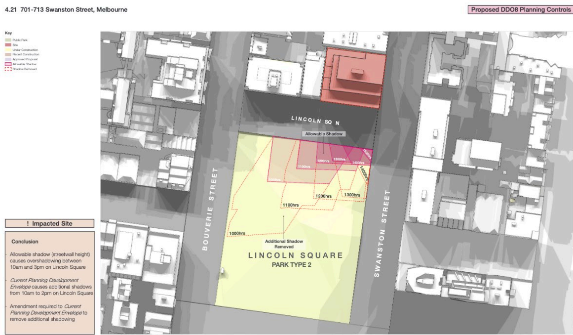
Figure 8 Extract from Mr Fulwood's built form testing demonstrating the extent of shadow at different times of the day
